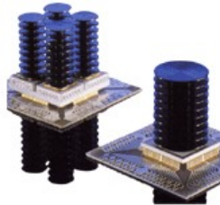
ECL (emitter-coupled -logic) LSI used by FACOM M-380, Left : 4K-bit RAM module with 5.5ns access time, Right : logic LSI with up to 1,300 or 400 gates
