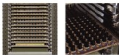
3D Stack, which can mount up to 13 MCCs and two side panels having newly developed ZIF (Zero Insertion Force) connectors for connecting signals between MCCs
