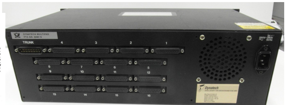
Figure 1. The Multi-PAD X.25 is often used with Dynatech's Multi-Switch X.25, which routes data from one X.25 trunk to another. Pictured here is an example of a large private data network incorporating Multi-Switch Model 12 and a number of Multi-PAD X.25s linking asynchronous terminals, hosts, and a public data network.
